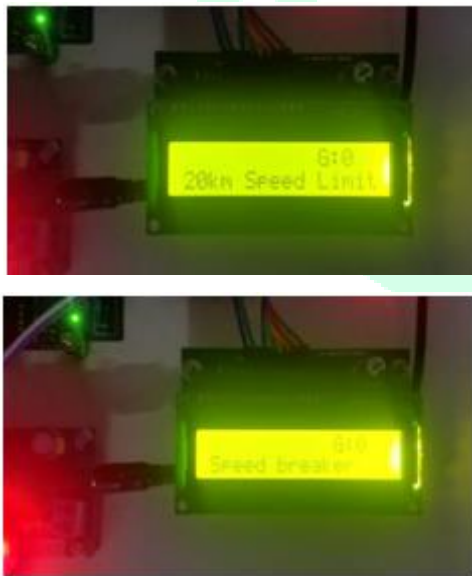
Fig 5: Sign board and Speed breaker detection
