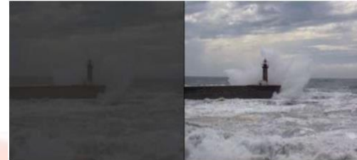
Fig. 1 The left image depicts the original image while the right picture shows the results after the normalization process. We can see that the original image is too dark while the normalized is not.
