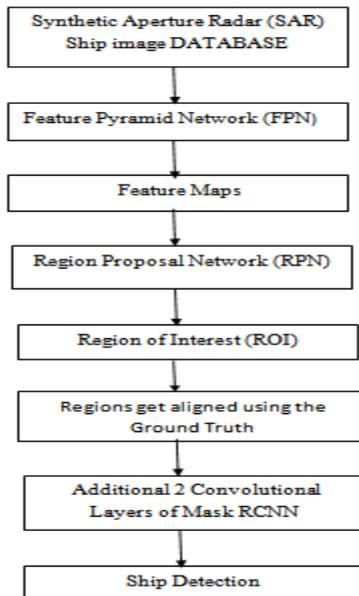
**Fig 1 steps for ship detection**
