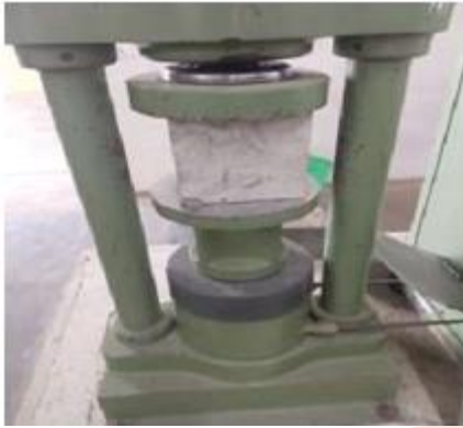
Fig 2: Compressive strength test and crack pattern
