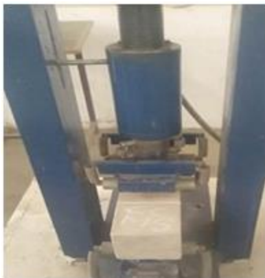
Fig 3: Split tensile strength test and crack pattern
