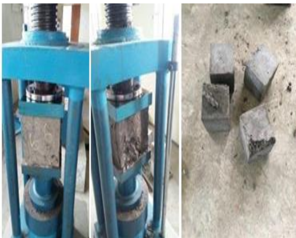
Fig 3: compression strength testing of conventional concrete
